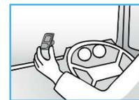
**Note:** Some windscreens have a metallic layer to reflect heat from the sun, In this case the tag must be placed within the designated areas of the windscreen without this coating. These are normally marked with a different color or pattern.
